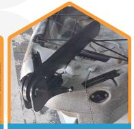
Set the rudder into the groove to ensure it is sitting in the center.
