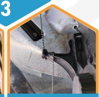
Wrap the remaining cord around the rudder assembly and tie it off.
