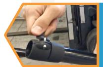
To tighten the paddle lock, Twist the paddle locking tab clockwise.
