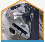
Insert the rudder into the steel ring at the back of the kayak.
