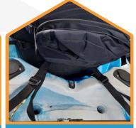
Connect the bottom two straps to the D-rings in the rear storage area.
