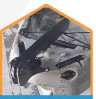
Set the rudder into the groove to ensure it is sitting in the center.
