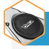
Featured on the Oceanus 12.5 fishing kayak is 2x water-resistant hatches. While only water-resistant they will handle the normal splashing that would occur when out on the water.
