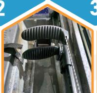
Pull the cord until the top of the foot pedal is in line with the bottom of the pedal.
