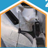
Feed the cord through the hole on either side of the rudder assembly.
