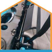
Using the bungee cord underneath the seat strap, loop the bungee cord over the clip.
