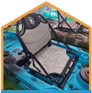
Place the seat in the allocated grooves.
