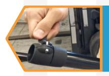
To tighten the paddle lock, Twist the paddle locking tab clockwise.
