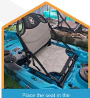
Place the seat in the allocated grooves.
