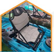
Place the seat in the allocated grooves.
