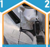
Feed the cord through the hole on either side of the rudder assembly.
