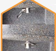
Secure the rudder onto the back with the included steel pin.
