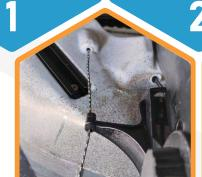
Feed the cord through the hole on either side of the rudder assembly.
