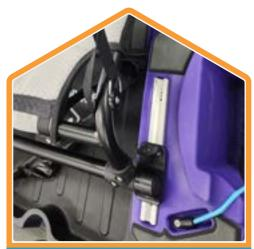
Alight the hole of seat adaptor/slidable fitting with the track nut's hole and use swing nut to fasten the seat.
