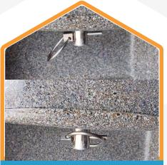
Secure the rudder onto the back with the included steel pin.
