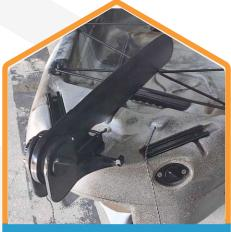
Set the rudder into the groove to ensure it is sitting in the center.
