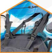
Connect the top two straps to the pad eyes on either side of the kayak
