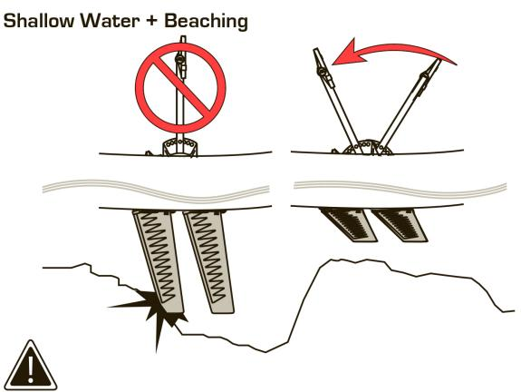
Press either pedal forward in shallow water to raise fins. Pressing one pedal fully forward will orient the fins with the kayak underside to allow beaching.
